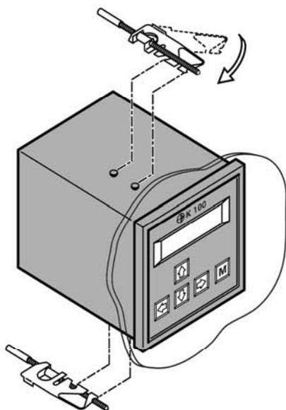
Install the instrument from the front side and fix it with the two mounting clips which were part of the delivery.
