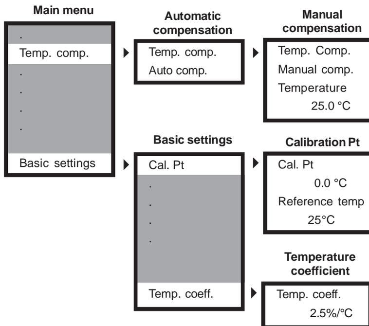
For automatic compensation you need a temperature sensor Pt100 (CM) or NTC (IL). All our conductivity sensors have integrated temperature sensors matching the instrument requirements.
