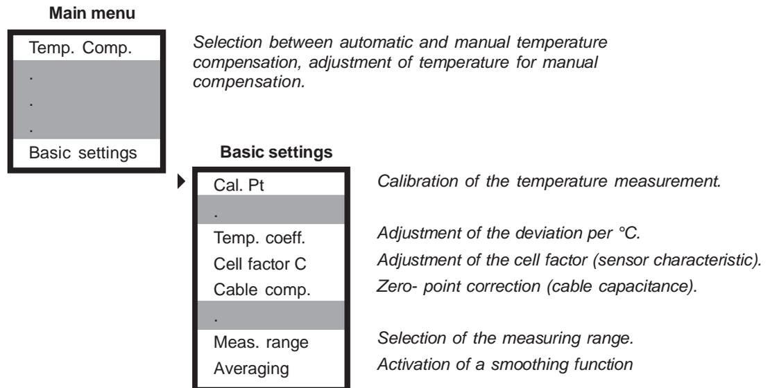
First choose the desired measuring range. Adjust the cell factor - it is indicated on the sensor. The cell factor accounts for the geometrical design of the sensor and allows to standardise the measured values.
